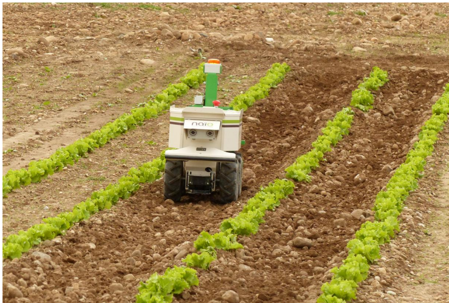
Figure 3: The weeding robot Oz. Source: Naïo Technologies.
