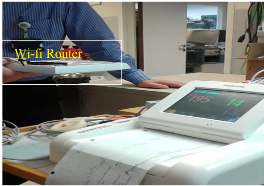
Fig. 1. The real-life example of EMI (CTG interference)
