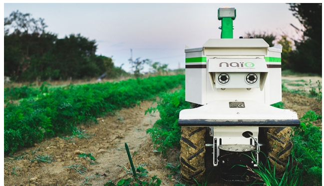
Fig. 2. The weeding robot Oz. Source: Naïo Technologies.
