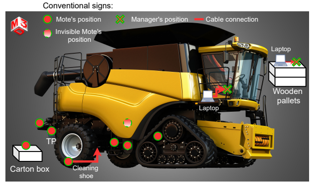
Fig. 4. SmartMesh IP test setup at CNHi
