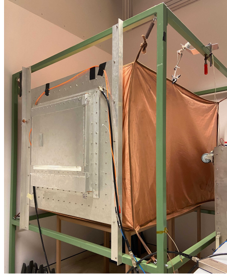
Fig. 1: An illustration of the VIRC setup used to mimic the hospital environment.
