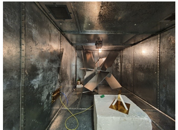
Fig. 3. Experimental setup inside the reverberation chamber showing Antenna 1 behind stirrer with PCB and Antenna 2 on polystyrene block.
